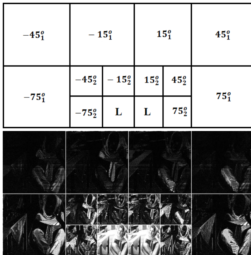
Figure 3.5: Improvement for directional features extraction in DT-DWT, Top: DT-DWT subbands at two decomposition levels, and bottom: DT-DWT transform of Barbara test image. Small coefficients are shown in black while large coefficients are shown in white.
