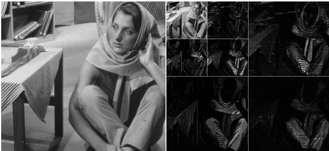
Figure 3.3: 2-D DWT. Left: Barbara test image and right: DWT using “db2” mother wavelet at two decomposition levels. Small coefficients are shown in black while large coefficients are shown in white
