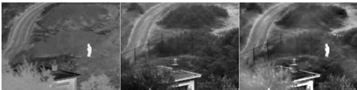
Figure 2.6: Fusion of multi-sensor images, from left to right: infrared and visible “UN Camp” images, and fused image.
