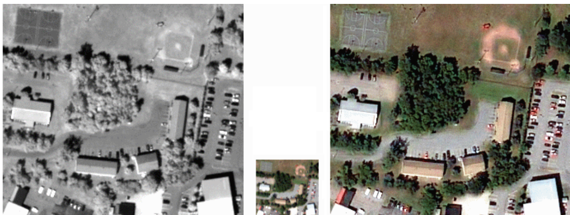
Figure 2.9: Remote sensing image fusion. Left to right: Pan, MS with lower resolution, and fused image (2004 Digital Globe).
