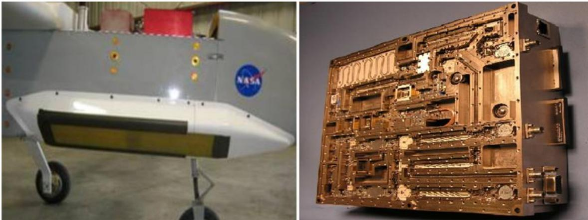
Figure 6.15: Left: Photograph of a microASAR system mounted on a small UAS, and right: SAR system hardware.
